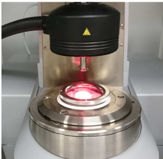
Figure S24. Photo of the rheometer with Intralipid containing agarose gel attached underneath the quartz plate. Red light ( 625\text{ nm} , 10\text{ mW cm}^{-1} ) can be seen passing through the phantom tissue.
